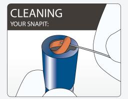
**4.** Clean your Snapit regularly. Remove O-ring as shown to disassemble the parts and clean with water or hospital grade cleaner. Do this in a clean dish to avoid loss of parts. Dry completely then re-assemble.
