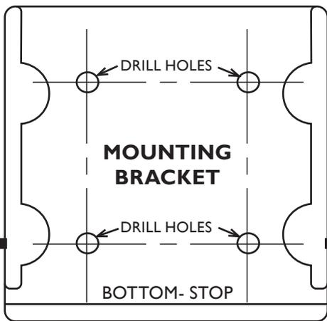
Adhere bracket with attached adhesive.
