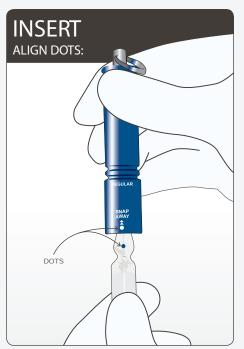
Align the dots if present. Gently insert all of the ampoule lit into the Snapit Lite. The ampoule lid becomes locked in at the neck.
